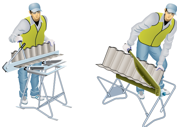
Figure 14.7.6.3 Ridge tile being bent then cut
