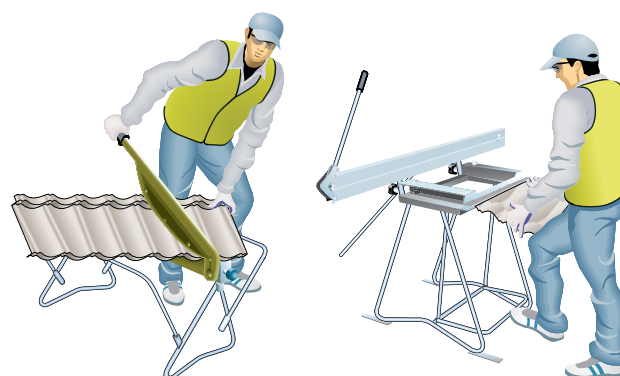
Figure 14.7.7.2 Valley tile being cut then bent
