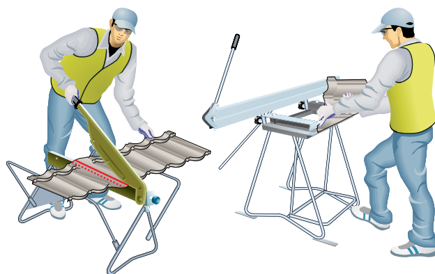
Figure 14.7.4.2 Gable end tile being cut then bent
