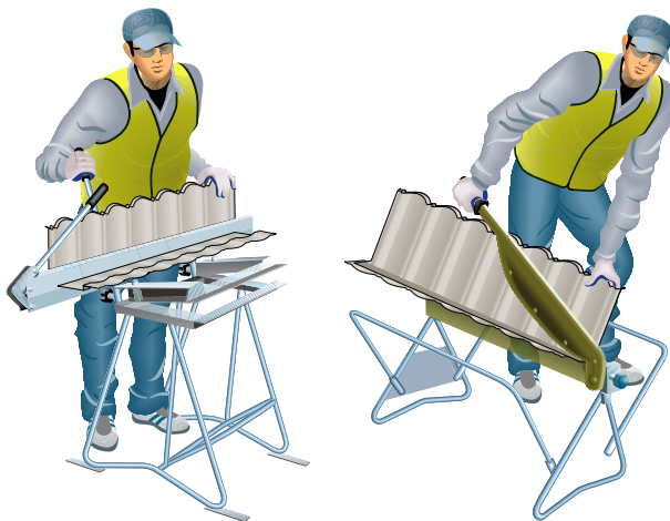
Figure 6.2.6.3 Ridge tile being bent then cut
