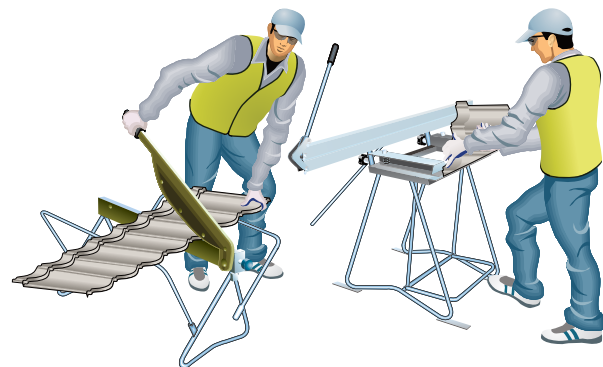
Fig 6.2.5.3 Hip tile being cut then bent
