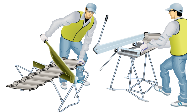
Figure 14.7.5.2 Cutting and bending a hip tile
