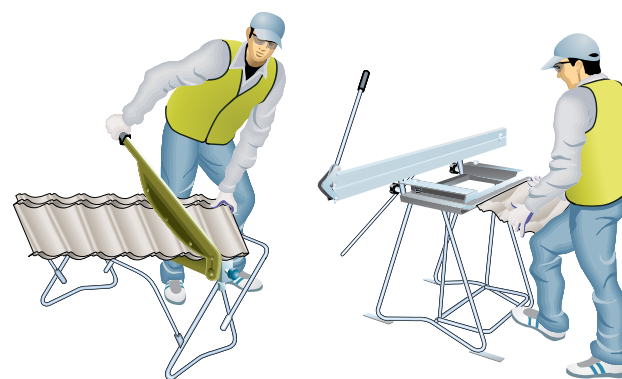
Figure 6.2.7.2 Valley tile being cut then bent
